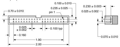
Figure 2. ATA interface connector
