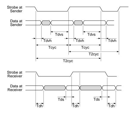
Figure 11. Sustained Synchronous DMA burst
