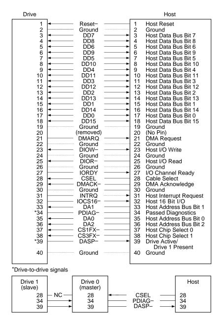
Figure 7. ATA interface connector pin assignments
