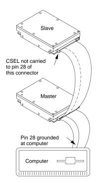
Figure 5. Connecting cable-selected drives
