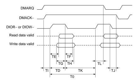
Figure 10. Multiword DMA timing
