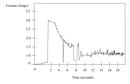
Figure 1. Typical startup current profile
