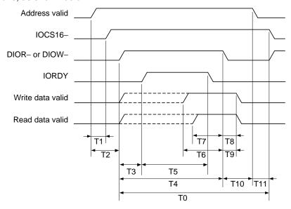
Figure 9. Programmed I/O timing with IORDY
