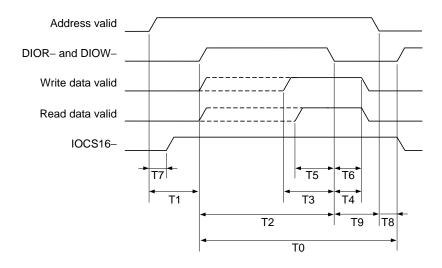
Figure 8. Programmed I/O timing without IORDY
